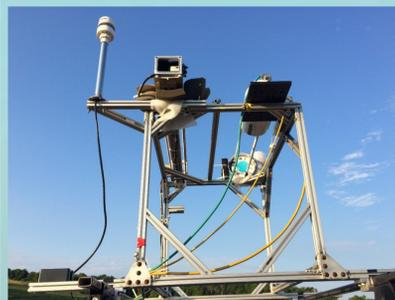
Figure 1: Mobile lab set up pictured. From left to right, AIRMAR, Ethane, Methane, CO<sub>2</sub>
