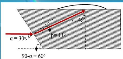
Fig. 1: In order to determine the optimum angles for a modified ZnSe prism, angles were found using the following derivation of Snell's Law: Given  $90 - (\alpha + \beta) = \gamma$ , and  $\beta = \arcsin(n_1/n_2 \sin(\alpha))$ , where  $n_1 = 1.00$  for air, and  $n_2 = 2.62$  for ZnSe.
