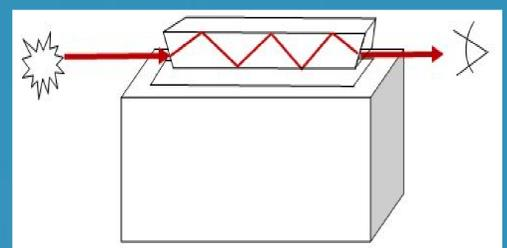
Fig. 2: This is the proposed modification to the traditional ATR-FTIR set-up, which normally utilizes two sets of mirrors. Here, the ZnSe prism can rest directly on a solid base, allowing the light to penetrate the crystal from the right side, and exit the crystal to be picked up by the detector on the left.
