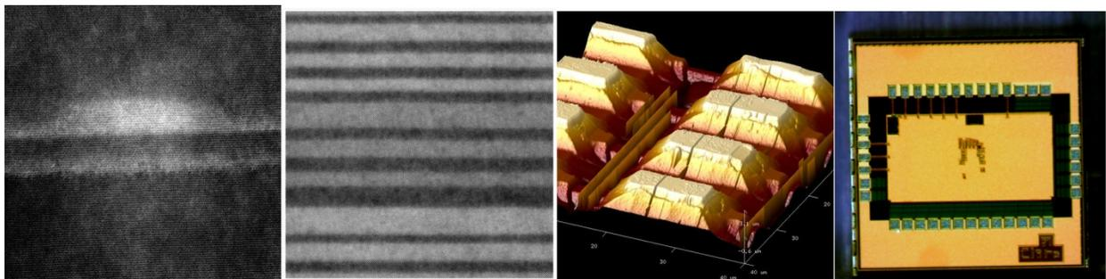
Figure 1: (from left to right) High-resolution transmission electron microscopy image of coupled InAs and InAlAs quantum dots (A, 40 nm x 40 nm) and of a low-noise QCD (B, 50 nm x 50 nm); Atomic force microscopy image of an array of pyramidally corrugated photodetectors (C, 40  $\mu\text{m}$  x 40  $\mu\text{m}$ ); 1.5 mm x 1.5 mm chip of a digital read-out circuit fabricated by TSMC using 0.18 $\mu\text{m}$  CMOS technology.
