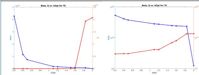
Beta is the attenuation factor, a unitless value representing the reduction in field strength as the mode propagates through the fiber. Q, the radiative quality factor, is relatively low for unguided modes, then increases substantially once the light line (a function of the refractive indices in the material) has been crossed. Q for guided modes is infinite in reality, and the large values above are computational approximations. All values above are for the fundamental mode.
